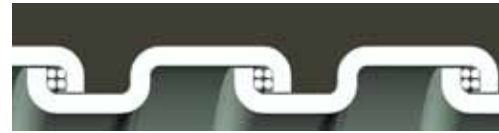
Square-Locked Design with cord packing 3/8" through 1-1/4"
